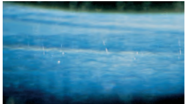
Figure 8. A wave-like appearance is visible on the planar surface between color bands in this 7.30 ct faceted synthetic pink quartz. The blue color is due to diffraction of light through the stone. Photomicrograph by Shane F. McClure; magnified 40 \times .
