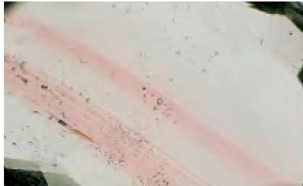
Figure 13. Curved planes of liquid and two-phase inclusions crossed the pink color bands at random angles in this natural pink quartz from Brazil. Photomicrograph by Shane F. McClure; magnified 10×.
