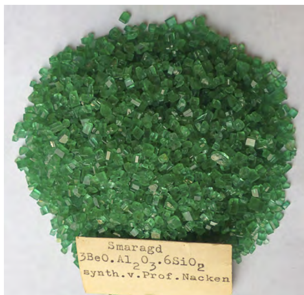
Figure 3. Synthetic emeralds produced by Nacken in the mid-1920s. Nacken left these and other samples to his family, and they are now in the possession of his grandsons. The label measures 45 × 23 mm. Photo courtesy of E. Schlatter.
