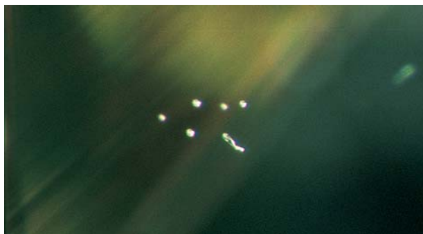
Figure 4. This group of gas bubbles is typical of Verneuil synthetic sapphire. Photomicrograph by Shane Elen; magnified 20 \times .
