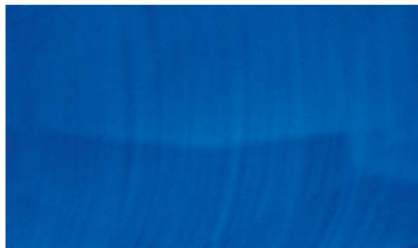
Figure 9. Curved striae cannot be detected in colorless synthetic sapphires with standard visible lighting. However, some flame-fusion synthetic sapphires may reveal this feature when exposed to SWUV radiation. Photomicrograph by Shane Elen; magnified 6x.
