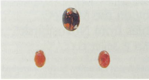
Fig.1. The new "hydrothermal" synthetic rubies reportedly from Novosibirsk. The colours observed are comparable to natural rubies from Thailand or Burma. Weights range from 1.69 ct to 0.62 ct.
