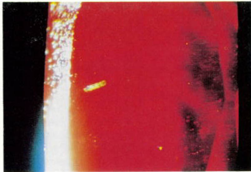
Fig.7. The highly reflective "golden" appearance of the copper alloy inclusions reaching the surface in a hydrothermal synthetic ruby is shown. (x45)
