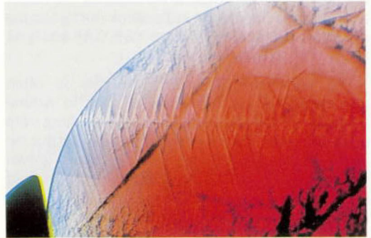
Fig.4. Unusual graining pattern in one of the "hydrothermal" synthetic rubies (0.62 ct), showing a "christmas tree" like image. The cause of this linear lattice disturbance is unknown. (x40)
